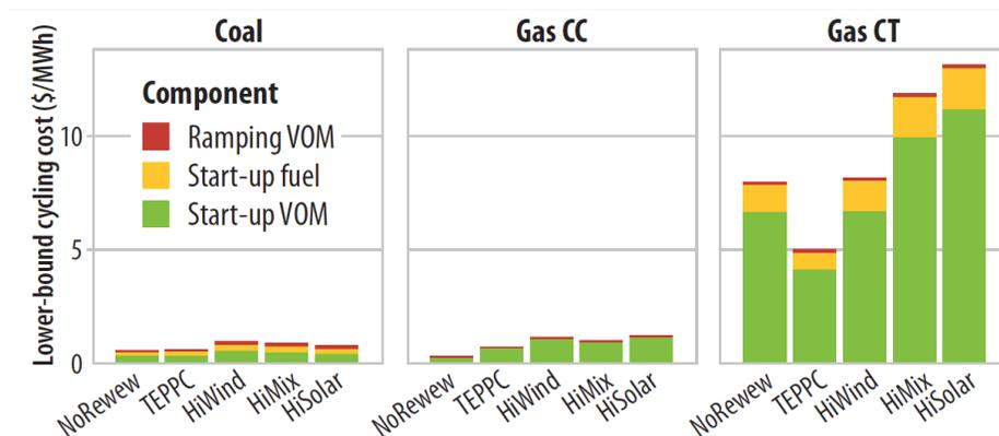
**Figure 1 – Lower Bound Cycling Maintenance Cost (The Western Wind and Solar Integration Study: The Effects of Wind and Solar - Induced Cycling on Wear-and-Tear Costs and Emissions 2013). Coal, Gas Combined Cycle, Gas CT**
